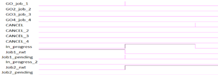
Fig. 6. Thread cancelled successfully for Use Case
