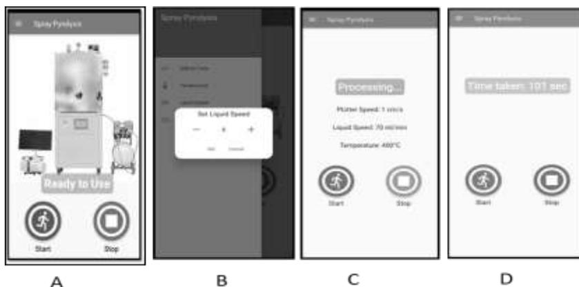
Fig. 6. a) Before the process, b) Set parameters, c) During process stage, and d) After the process
