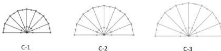
**Fig. 9.** Crack-tip modeling by configuration of size of elements
