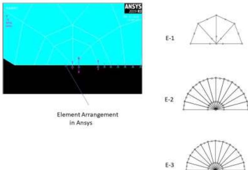
**Fig. 8.** Crack-tip modeling by configuration of number of elements
