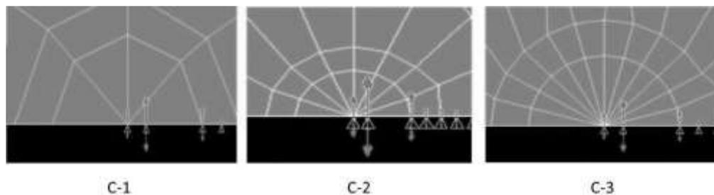
**Fig. 12.** Angular discretization at crack tip
