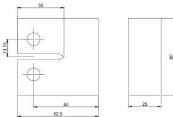
**Fig. 5.** Compact testing specimen according to the ASTM E 399 standard [11]
