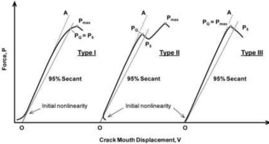
Fig. 4. Principal Types of Force-Displacement (CMOD) Records
