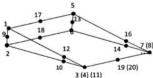
Fig. 2. Singular pentahedral element
