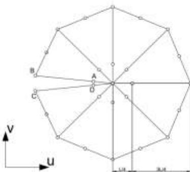
**Fig. 6.** SINGULAR element around the crack tip
