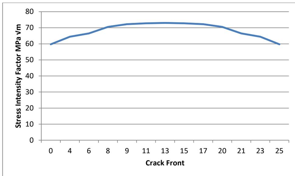
**Fig. 13.** Variation of SIF along the crack edge.
