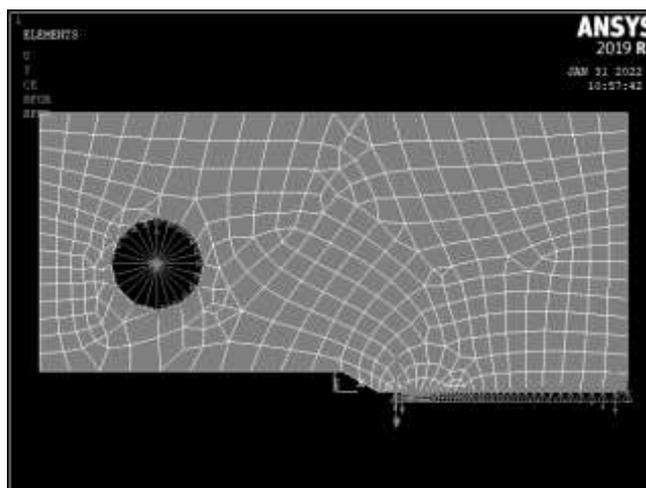
Fig. 7. Mesh, Loading and boundary conditions.
