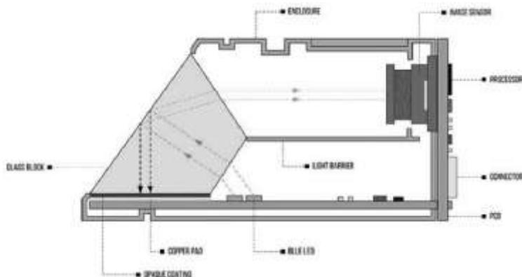
Fig. 1. Schematic of R307 Fingerprint Sensor
