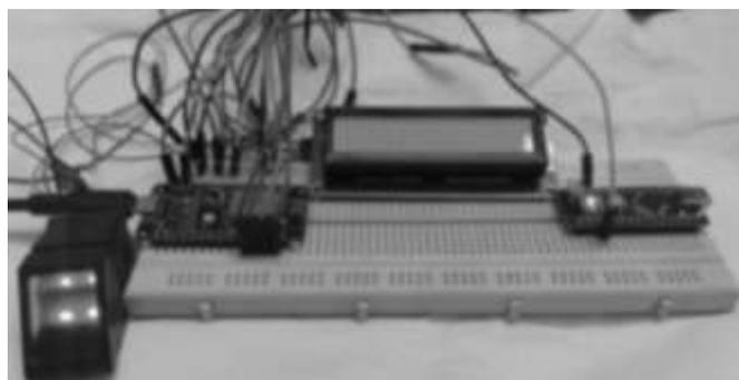
**Fig. 3.** Biometric Attendance System Using Fingerprint Sensor
