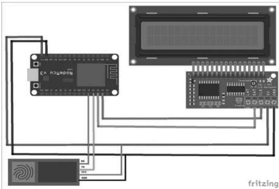
Fig. 2. Fritzing Diagram of Biometric module
